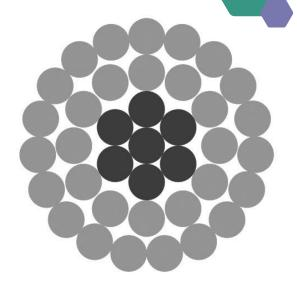
Steel Galvanized wires for ACSR manufacturing. ASTM standards
